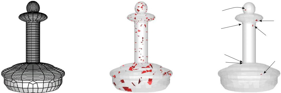
Figure 2: PAWN: input (left), slivers before PUMP (middle), few slivers survive PUMP (right). Most of the input face angles close to \frac{\pi}{2} on the boundary are evaluated as acute for numerical tolerances. All surviving slivers are near some such acute angles.
