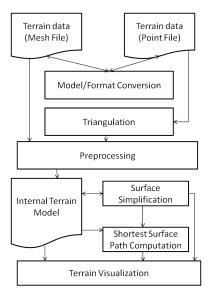
Figure 2: Architecture of Terrain-Toolkit
