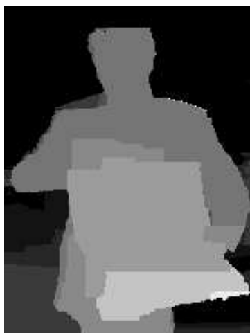
Fig. 16. Disparity map computed with the method of Kolmogorov et al. [1] on the same sequence as Figure 14.
