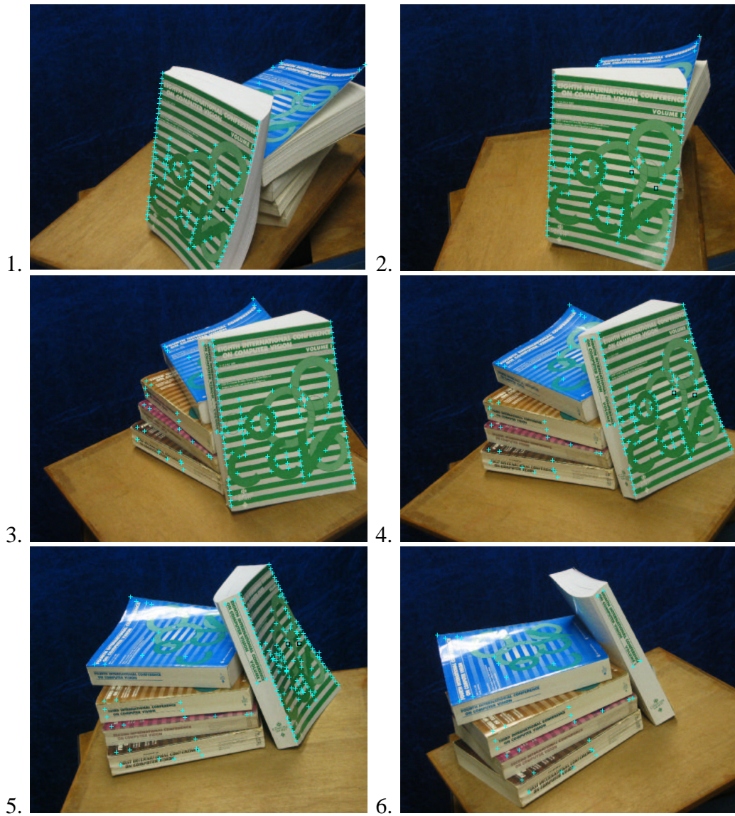
Figure 8: The six images of the proceedings captured at different positions and the corresponding points of interest. The square marks in the images 1, 2, 4, and 5 are the minimal data selected by RANSAC.
