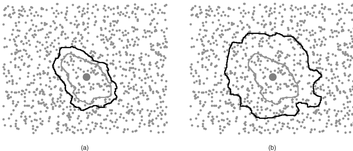
Fig. 6. A flexible variant for constraining broadcasting. (a) Influenced area for a small TTL value. (b) Influenced area for a large TTL value.
