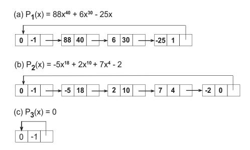
You must use the three classes Node, ListIterator, and List (should be modified to adapt the change to circular structure) covered in class to do the job:
