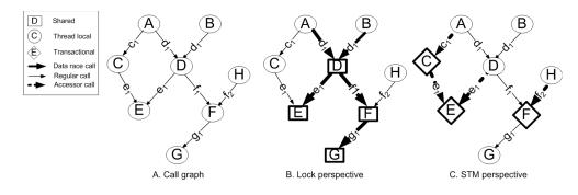
Figure 2. Synchronization perspectives of the call graph
