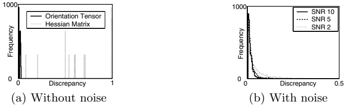
Fig. 2. Orientation discrepancies between the estimated and the truth flow iso-surface normals. (a) Without noise; (b) with noise, the orientation tensor approach only
