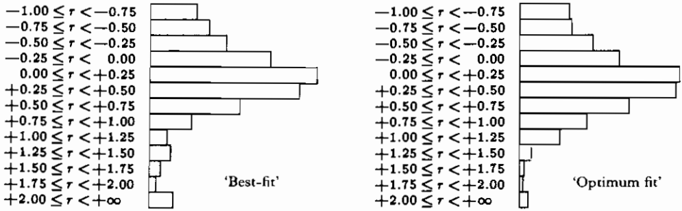
Figure 20. The distribution of interword spaces found by the best line-at-a-time method, compared to the distribution found by the best paragraph-at-a-time method, when difficult mathematical copy is typeset without human intervention.
