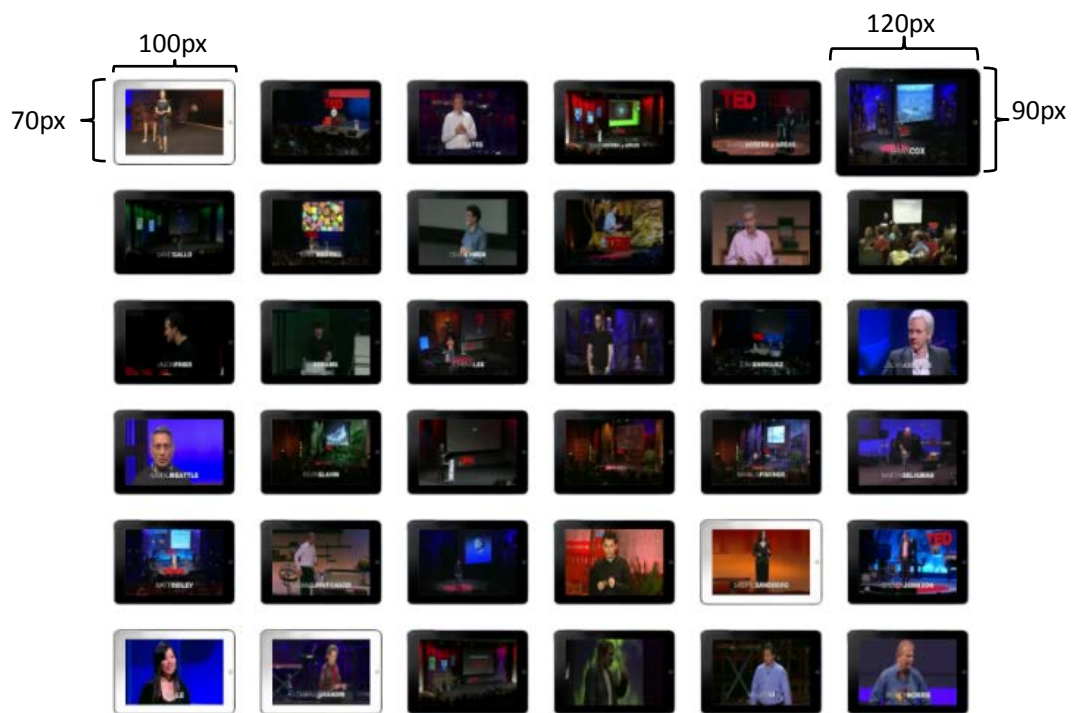
(b) Retrieve individual tiles by transforming a video buffer to 36 blocks
