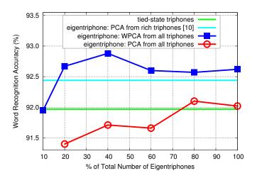
Fig. 1. Effect of weighted PCA and eigentriphone pruning using bigram LM.
