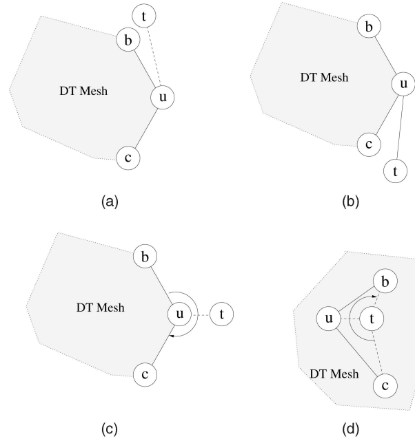
Fig. 4. (a), (b), and (c) Host u is on the boundary of the overlay mesh, and host t lies outside the mesh. (d) u is an interior host of the mesh. Host t lies inside triangle \triangle abc , but does not belong to the mesh.
