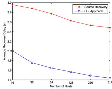
(a) Average recovery delay versus the number of hosts as compared with source recovery.
