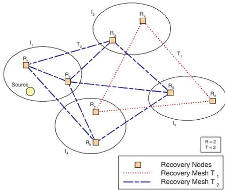
Fig. 1. Illustration of constructing recovery meshes.
