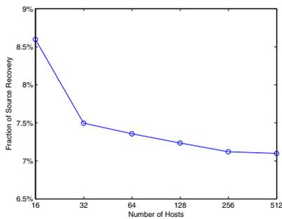
Fig. 7. Fraction of source recovery used in our retransmission scheme.
