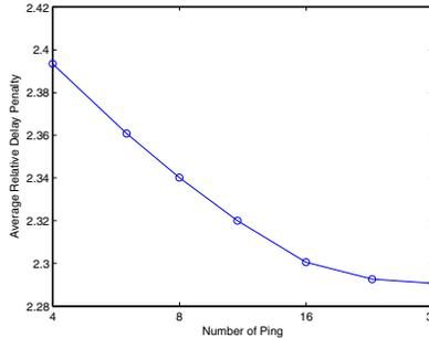
Fig. 3. Average RDP versus the number of ping measurements for our approach.
