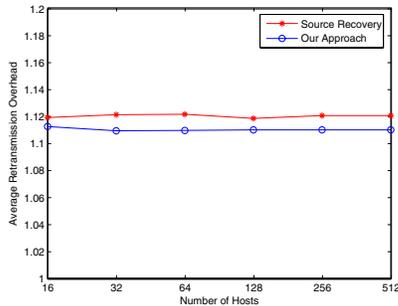
Fig. 6. Average retransmission overhead per lost packet versus number of hosts.
