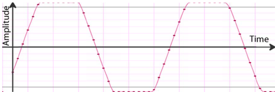
Figure 6.1: Illustration of the clipping problem. The clipped samples are the points that appear to be "attached to" the top and bottom. The grey lines are safe bounds for software playback, the top and bottom lines are hardware boundaries during the recording
