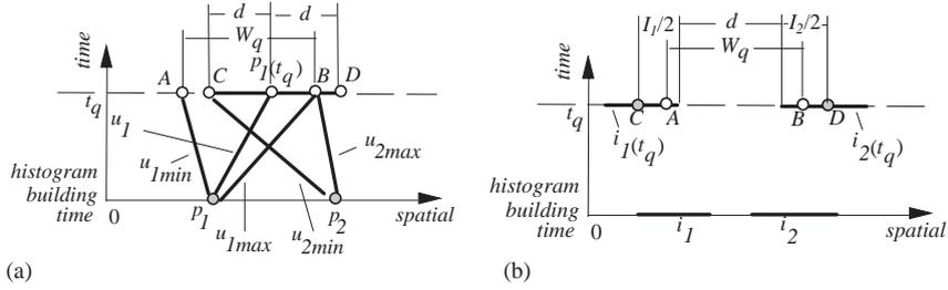
Fig. 9. Analysis of constrained joins. (a) Deriving  $P_{C-pair}(l_1, l_2, u_1, W_q)$  for point data, (b) a pair of qualifying intervals.
