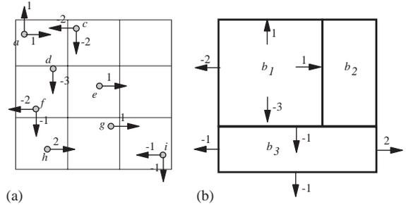
Fig. 3. A spatio-temporal histogram. (a) Object location and velocities, (b) the final buckets.
