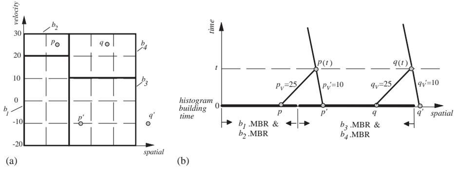
Fig. 13. Updating the histogram. (a) The cells and buckets, (b) point  $p$  falls in a different bucket after update.
