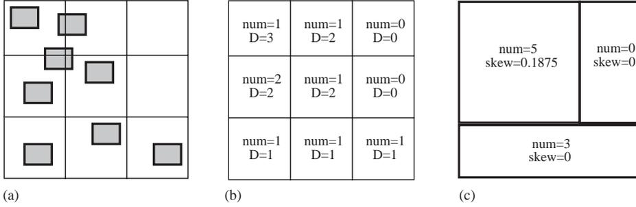
Fig. 2. Building the histogram. (a) 3 × 3 grid, (b) cell information, (c) the final buckets.
