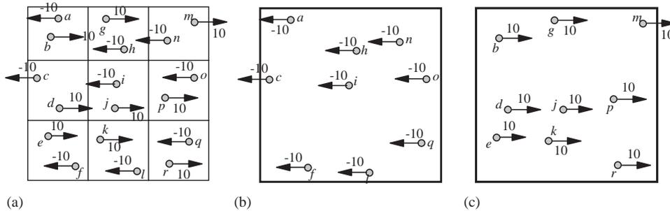
Fig. 12. Skewed velocity distribution. (a) Cell information, (b) bucket 1, (c) bucket 2.
