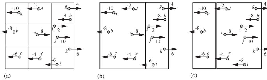
Fig. 11. Uniform velocity distribution. (a) Cell information, (b) considering only location, (c) location and velocity.
